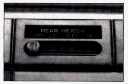
You may have the optional rear heater. The three speed fan switch is above the radio. Slide the lever toward HI for warmer air in the rear area. Move the switch to OFF to turn the system off.
